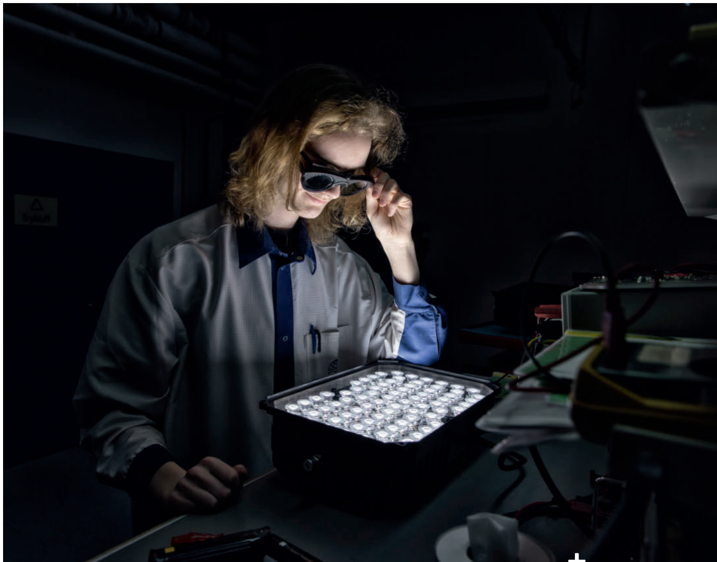
GPV subjects its products to a number of quality tests during the production process. This picture shows a visual inspection of high-performance LED units.
