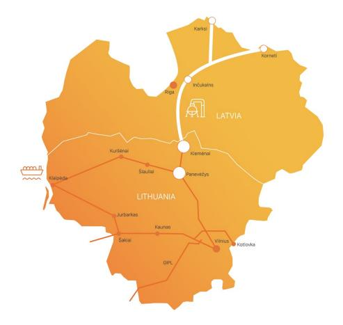
The project's implementation in the territory of Lithuania will cover capacity enhancement of Kiemėnai gas metering station and reconstruction of the gas pipeline at Panevėžys gas compressor station. The project's implementation in the territory of Latvia will cover reconstruction of the main gas pipeline in order to increase the maximum working pressure from 40 to 50 bar.
